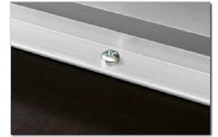
Triple securing system of the panel to the frame: Aluminium rivets, stainless steel screws on the underside of the frame and silicone sealed.
