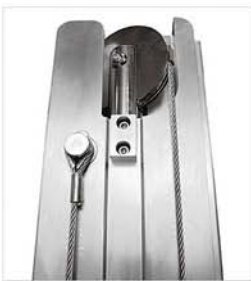
Reinforced Aluminium Sections (EN-AW 6082 T6). Special galvanised non-rotating steel wire rope with steel core. Construction: 19x7+0
